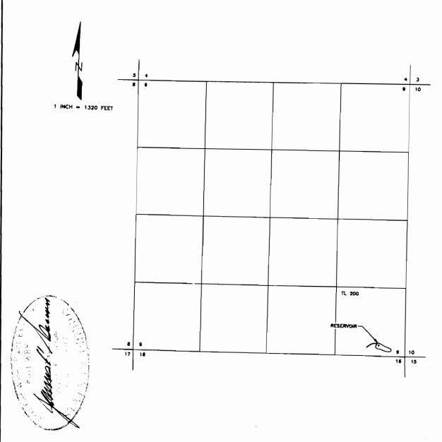
THE RESERVOIR IS LOCATED 150 FEET NORTH AND 400 FEET WEST FROM THE SOUTHEAST CORNER OF SECTION 9, BEING WITHIN THE SE 1/4 SE 1/4 OF SECTION 9, TOWNSHIP 24 SOUTH, RANGE 6 WEST, W.M., DOUGLAS COUNTY.
