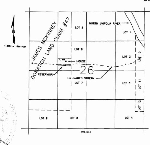
THE DAM IS LOCATED 2430 FEET SOUTH AND 1560 FEET EAST FROM THE NORTHWEST CORNER OF SECTION 26, BEING WITHIN THE SE1/4 NW1/4 SECTION 26, TOWNSHIP 26 SOUTH, RANGE 6 WEST, W.M., DOUGLAS COUNTY.
