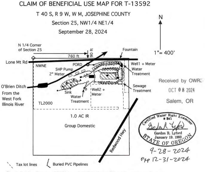
Point of re-diversion (PORD) from the O'Brien Ditch, 5 HP pump, and 2" water meter. The PORD is 90 feet south and 760 feet east from the north 1/4 corner of Section 25. The POD on the West Fork Illinois River and the ODFW fish screen are shown on the transfer map.
