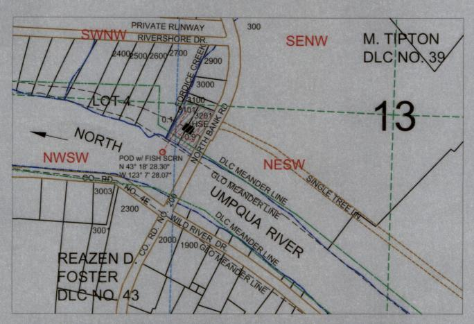
POD IS LOCATED 297 FEET SOUTH & 1380 FEET WEST OF C1/4 CORNER OF SECTION 13.
