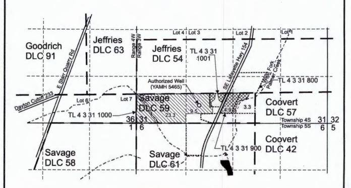
Authorized Well (YAMH 5465) is located 501 feet north and 1,772 feet east from the SW corner, Section 31.
