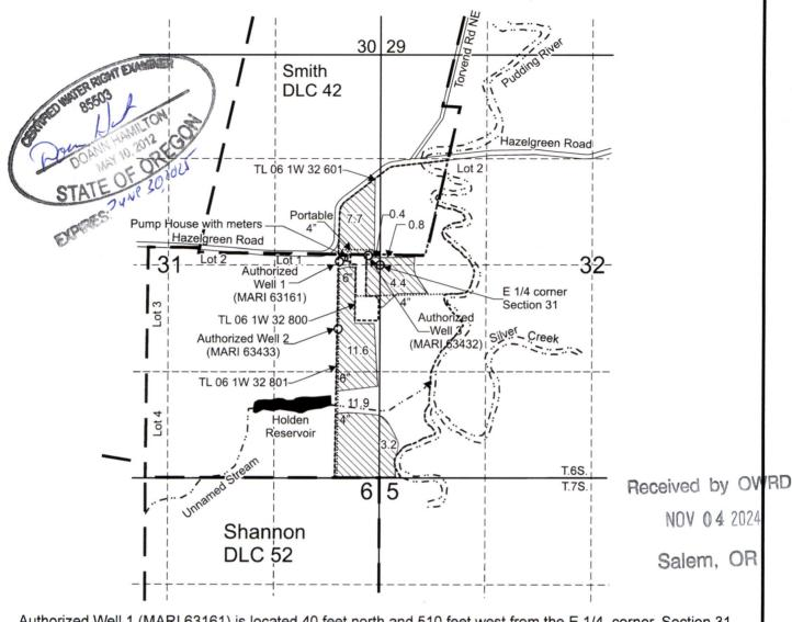
Authorized Well 1 (MARI 63161) is located 40 feet north and 510 feet west from the E 1/4 corner, Section 31. Authorized Well 2 (MARI 63433) is located 800 feet south and 520 feet west from the E 1/4 corner, Section 31. Authorized Well 3 (MARI 63432) is located 110 feet north and 150 feet west from the E 1/4 corner, Section 31.
