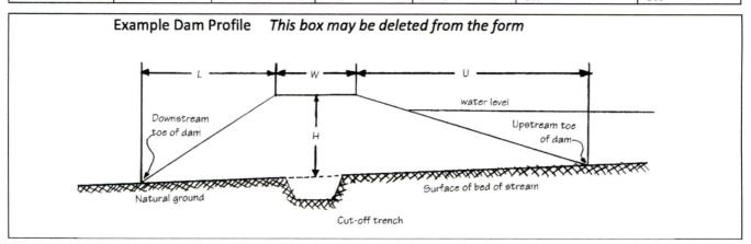
6. Provide a drawing showing the cross section of the dam at the maximum section indicating details and dimensions. The drawing should be drawn at a standard even scale.
