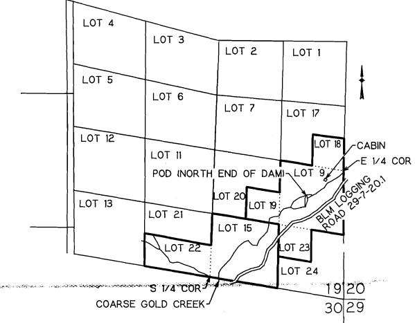
POD (NORTH END OF DAM) IS 480 FT S AND 740 FT W FROM E 1/4 COR SEC 19 SEE DETAIL MAP FOR STATEMENT CONCERNING ADDITIONAL POD'S AND PLACES OF USE
