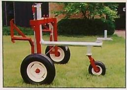
Row Crop Gun Cart with galvanized body is standard equipment. An optional Low Profile Gun Cart is also available.
