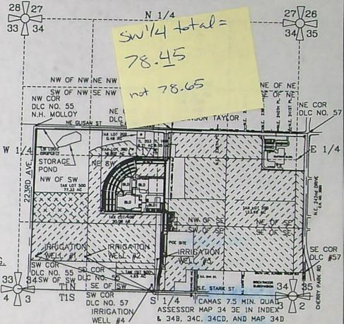
IRRIG. WELL #1 IS LOCATED 710 FEET NORTH AND 2280 FEET WEST IRRIG. WELL #2 IS LOCATED 700 FEET NORTH AND 1335 FEET WEST IRRIG. WELL #3 IS LOCATED 650 FEET NORTH AND 60 FEET EAST IRRIG. WELL #4 IS LOCATED 150 FEET NORTH AND 50 FEET WEST OF THE SOUTHEAST QUARTER CORNER OF SEC. 34. WELLS #1, #2 & #4 ARE LOCATED IN THE SW 1/4 AND WELL #3 IS LOCATED IN THE SOUTHEAST 1/4 OF SECTION 34, TOWNSHIP 1 NORTH AND RANGE 3 EAST of the WM, MULTNOMAH COUNTY, OREGON
