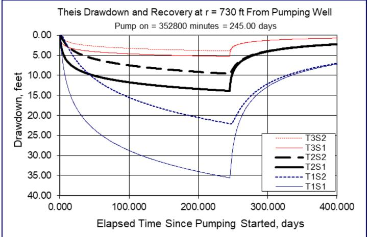
Radial distance from pumping well (r)=730 ft [estimated radial distance to nearest user, 16361 NW Red Shot Lane, TL 400] **Pumping Rate (Q)= 0.0557 cfs (~25 gpm)**
