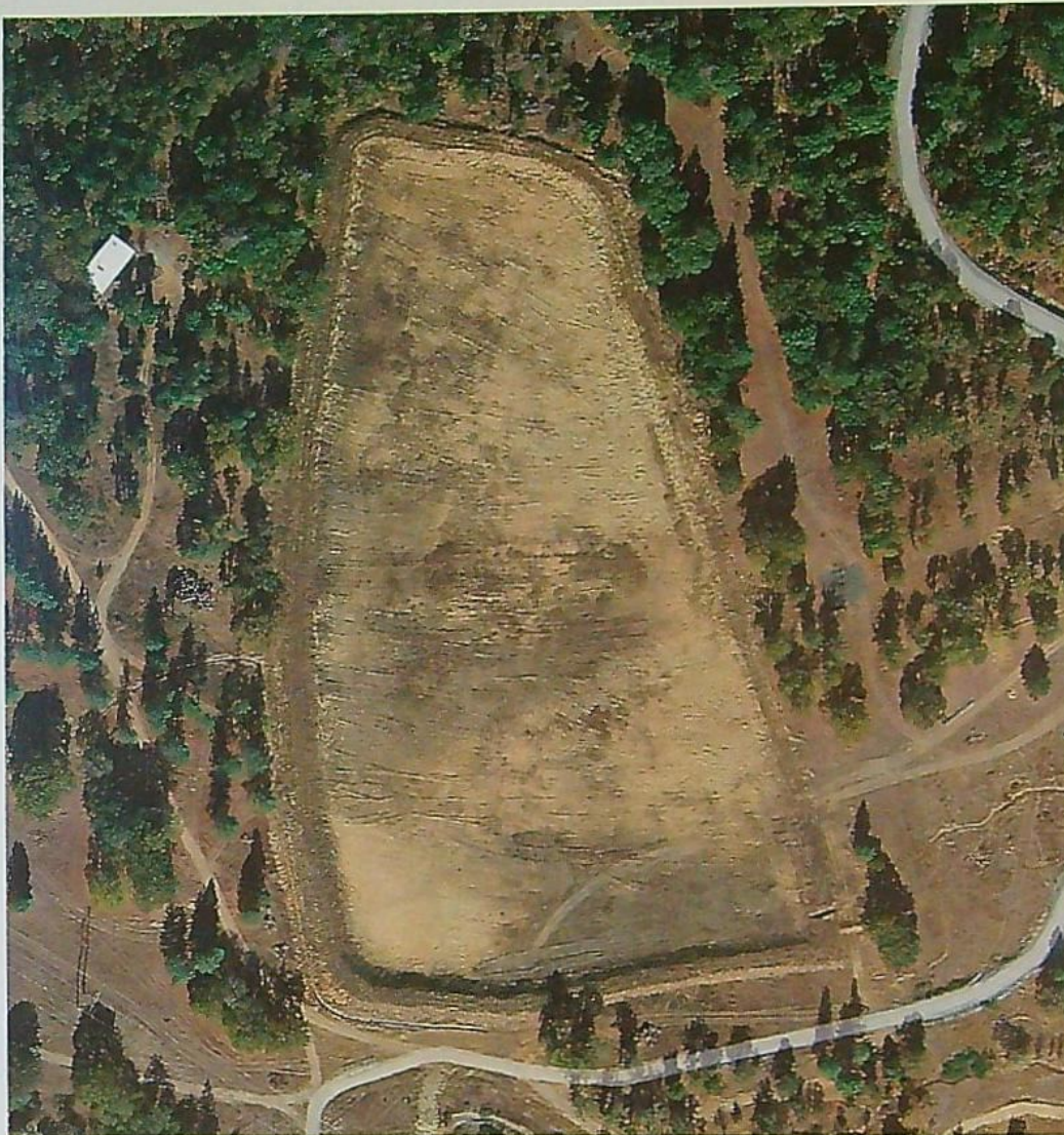
Aerial image showing construction of Reservoir #4, including the berm around the reservoir.
