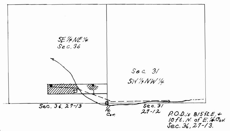
Storage Reservoir at P.O.D. is 2,000 gal. Pipe is 1/4"Dia. Dam is 1/3 ft. high + 16ft. long.
