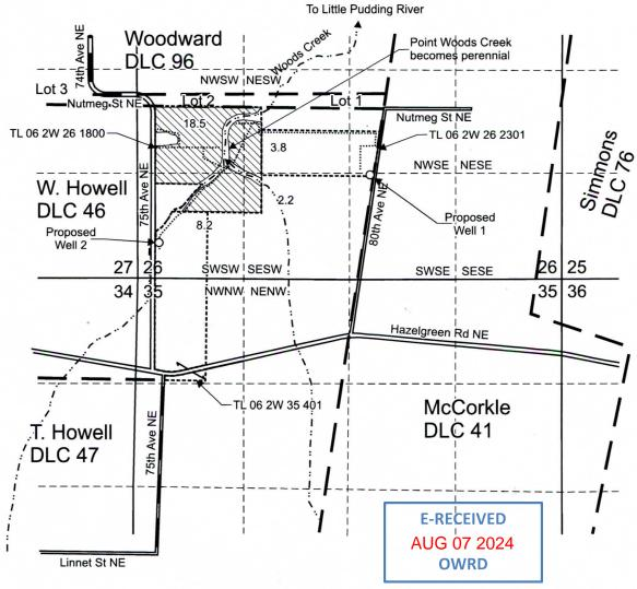
Proposed Well 1 is located 1,310 feet north and 2,380 feet west from the SE corner, Section 26. Proposed Well 2 is located 445 feet north and 265 feet east from the SW corner, Section 26.
