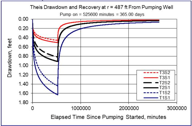
Radial distance from pumping well (r)=487 ft [estimated radial distance to nearest user, MARI 4801] **Pumping Rate (Q)= 0.61 cfs (273.8 gpm)**
