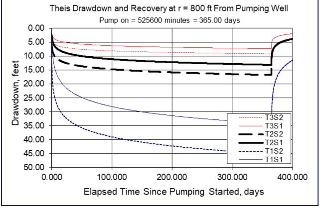
Radial distance from pumping well (r)=800 ft [estimated radial distance to nearest user, MARI 6511] **Pumping Rate (Q)= 0.74 cfs (~333.85 gpm)\***
