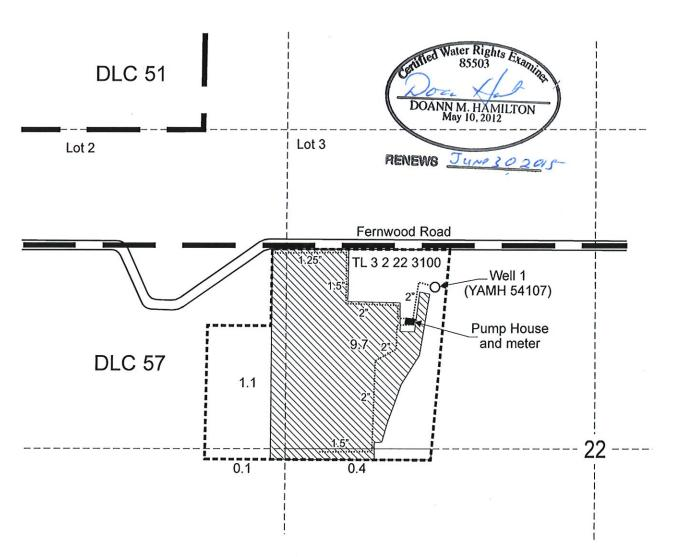
Well 1 is located 650 feet south and 970 feet east from the SE corner, DLC 51.
