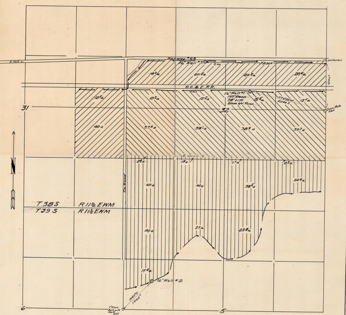
I, W.R. CANTON, of Klomoth Folls Oregon do hereby certify that, this map was made from notes Taken during an actual survey mode by me on April 1, 1948; that the monuments shown on this map consisting of a ford axle was set on the Section line athe 1/4 corner common to Sections 32 + 33 T 385, R 11/2 E.W.M. and a 1" iron bolt with nut attached was set at the 1/4 Corner common to Sections 5 and 6 T 395 R 11/2 E.W.M in Klamath County Oregon.
