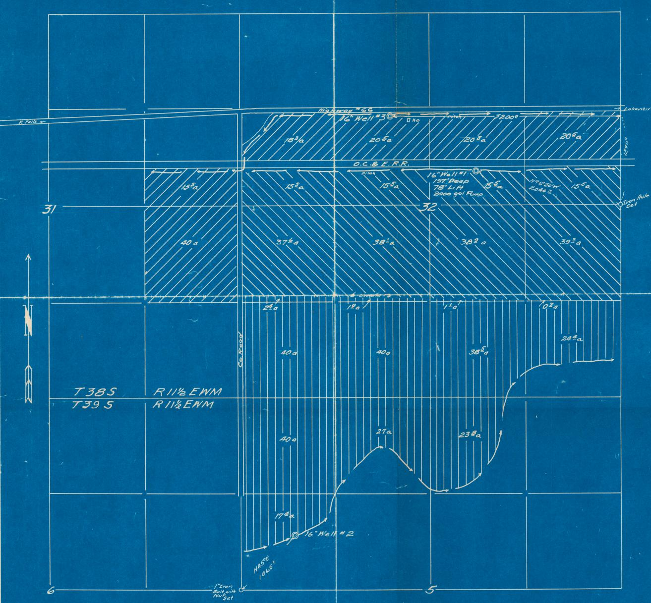
I, W.R. CANTON, of Klomoth Folls Oregon do hereby certify that, this map was made from notes Taken during an actual survey mode by me on April 1, 1948; that the monuments shown on this map consisting of a ford axle was set on the Section line athe 14 corner common to Sections 32 + 33 T 385, R 11/2 E.W.M. and a l"iron bolt with nut attached was set at the 1/4 Corner common to Sections 5 and 6 T 395 R 11/2 E.W.M. in Klamath County Oregon.
