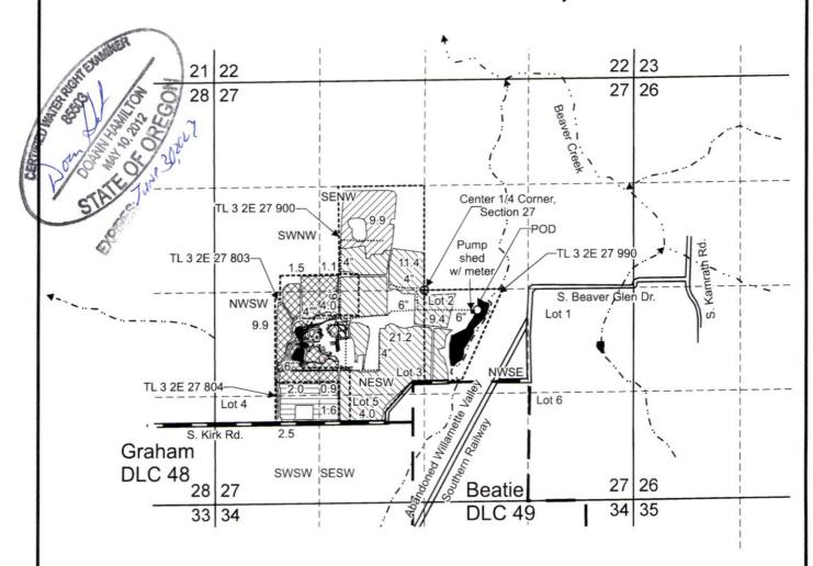
POD is located 240 feet south and 665 feet east from Center 1/4 corner, Section 27.
