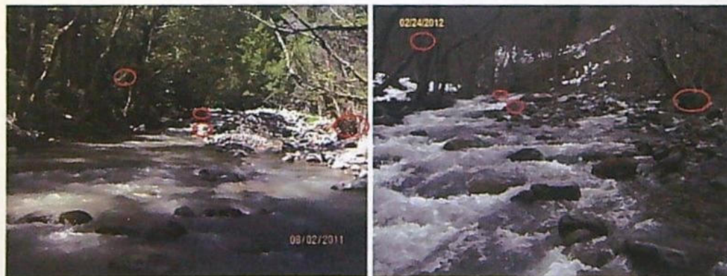
Figure 11. Channel change at Transects 1-3 (scour at downstream end at Transect 1; aggradation at upstream end on Transect 3) between August, 2011 and February, 2012 (looking upstream).
