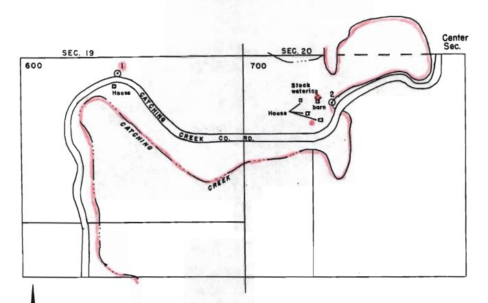
Point of diversion I is located N85°35'E a distance of 4133' from the center section.
