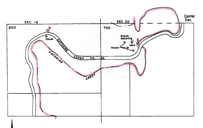
Point of diversion I is located N85°35'E a distance of 4133' from the center section.
