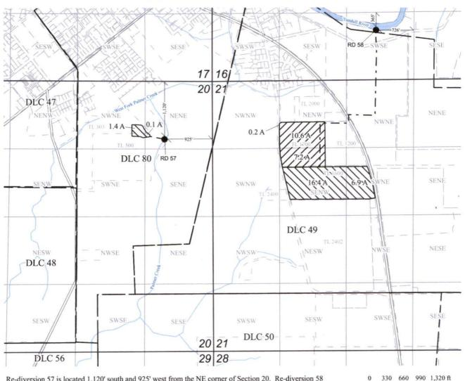
Re-diversion 57 is located 1,120' south and 925' west from the NE corner of Section 20. Re-diversion 58 is located 365' south and 726 west from the NE corner of SW1/4 SE1/4 of Section 16. PCWDIC POD is located 4,700' north and 1,290' east from SE corner of DLC 58 (see Map 6 of 6).
