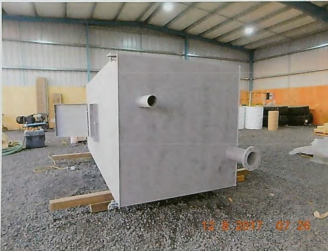
PHOTO 4 Fabrication of spring box
