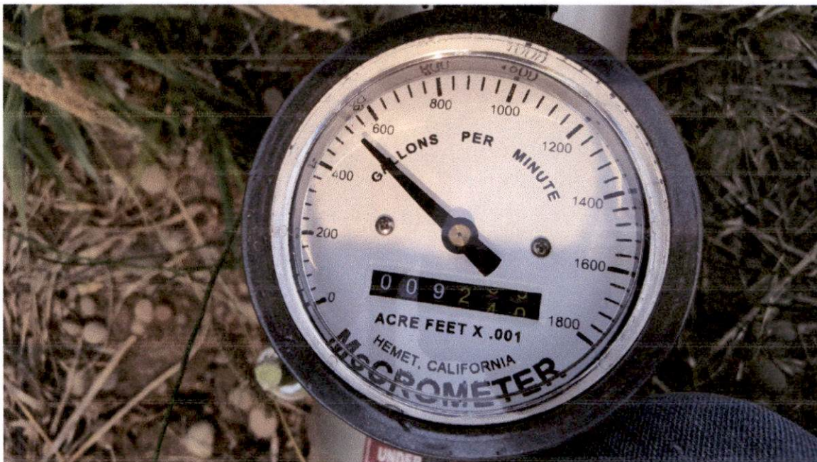
Photo 2: Meter showing starting volume in acre feet and flow rate is gpm.
