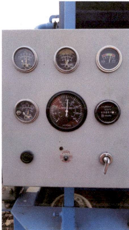
Photo 10: Engine/Pump instrument panel.
