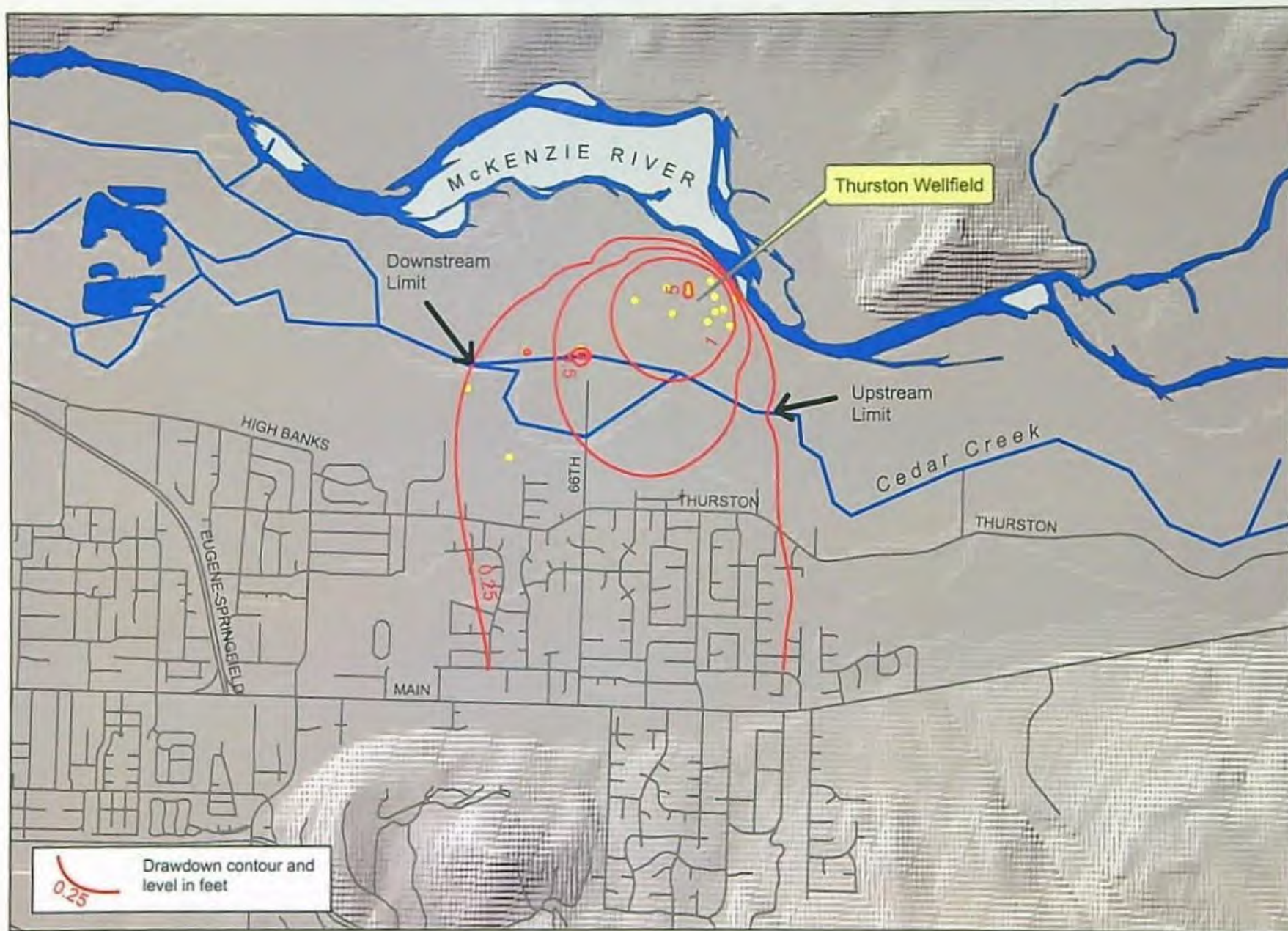
Figure 2 Modeled Incremental Drawdown without Cedar Creek Flow
