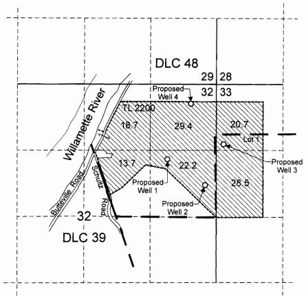
Proposed Well 1 is located 1,500 feet south and 970 feet west from the NE corner of Section 32. Proposed Well 2 is located 2,020 feet south and 220 feet west from the NE corner of Section 32. Proposed Well 3 is located 1,200 feet south and 150 feet east from the NW corner of Section 33. Proposed Well 4 is located 390 feet south and 510 feet west from the NE corner of Section 32.
