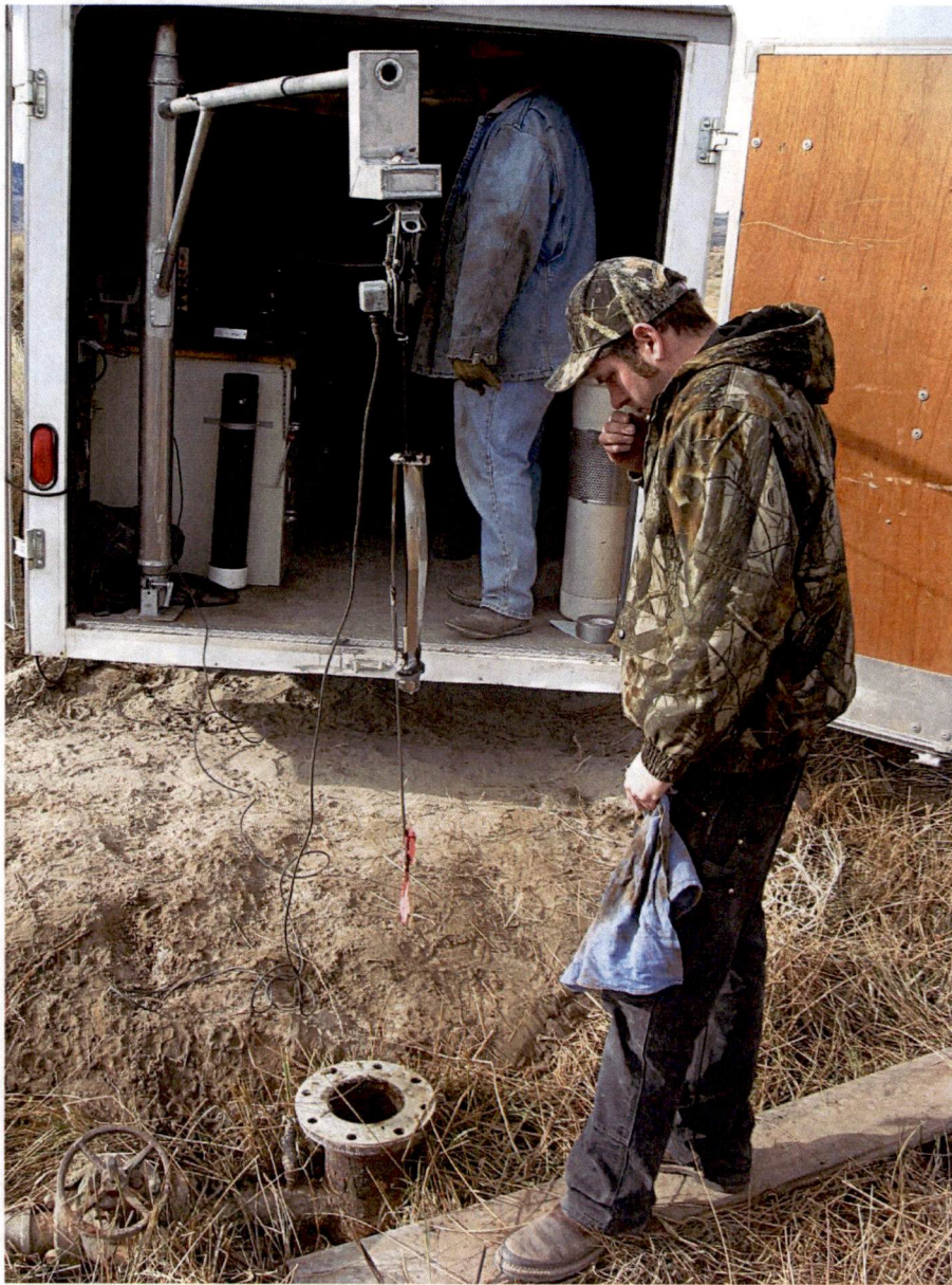
Figure 3. Camera down Saddoris Well (Well 1) January 16, 2012.
