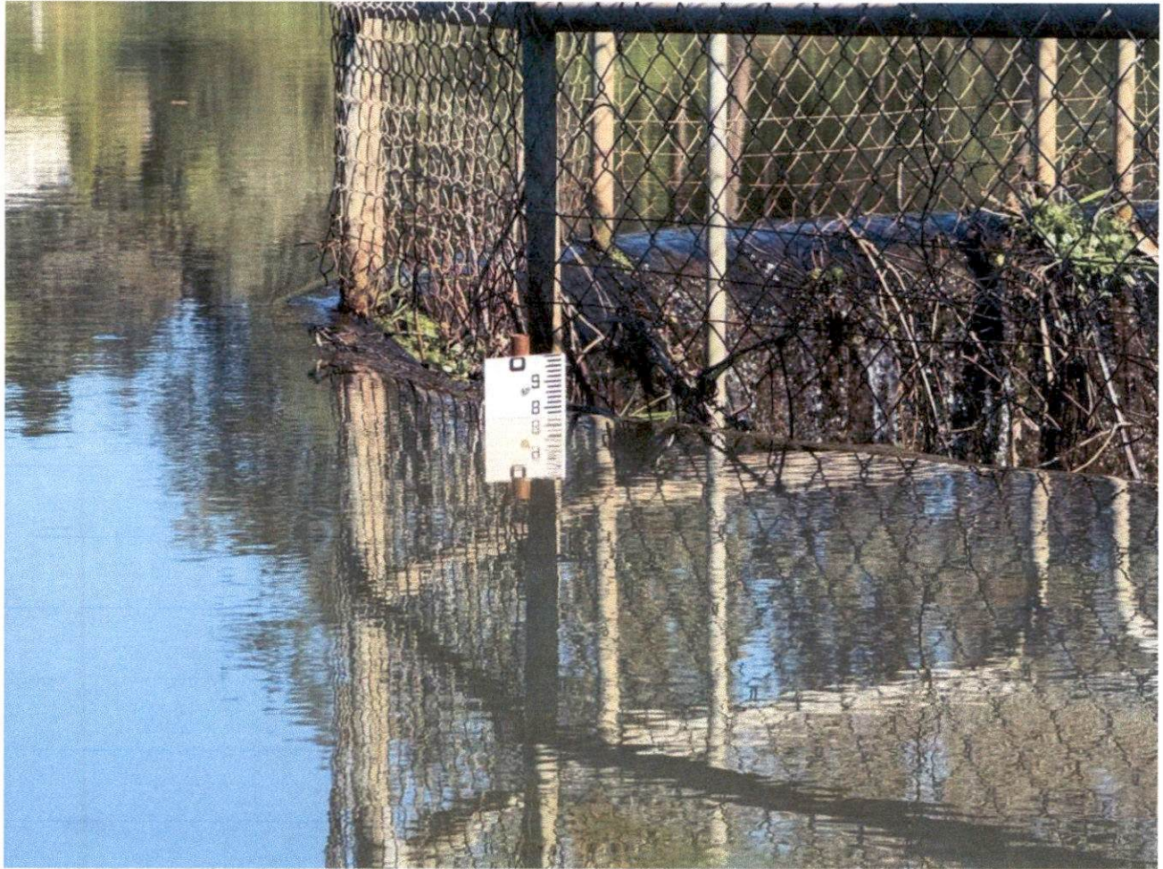
Installed Staff Gage on April 18, 2025
