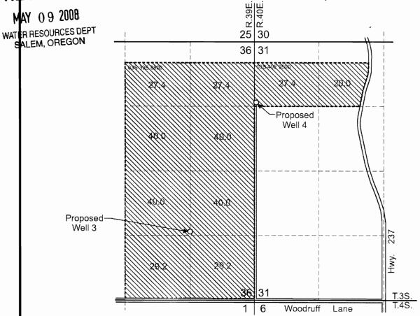
Proposed Well 3 is located 1,400 feet north and 1,320 feet west from the SE corner, Section 36. Proposed Well 4 is located 1,400 feet north and 36 feet east from the W1/4 corner, Section 31.
