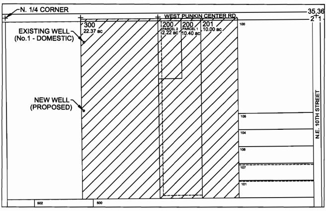
EXISTING DOMESTIC WELL LOCATED 200' SOUTH & 660' EAST OF N 1/4 CORNER OF SECTION 2. PROPOSED IRRIGATION WELL TO BE LOCATED 770' SOUTH & 660' EAST OF N 1/4 CORNER OF SECTION 2.
