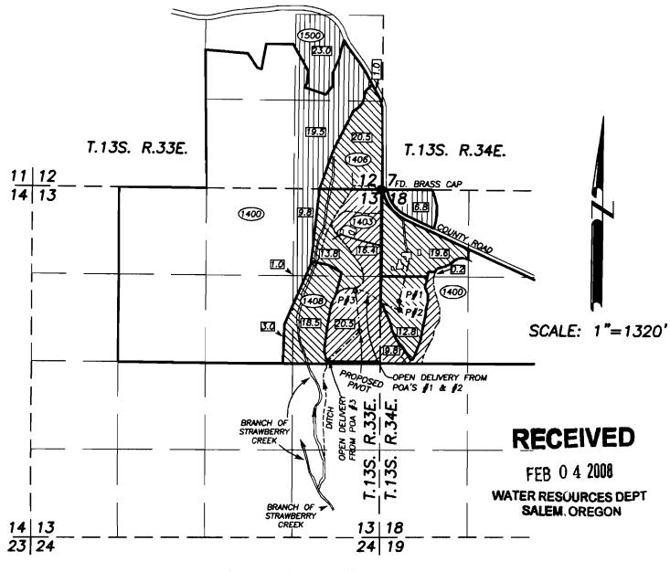
EXISTING WELL AT PROPOSED POA #1 IS 1695' S. & 280' E. OF THE NW COR. SEC. 18, T.13S., R.34E, EXISTING WELL AT PROPOSED POA #2 IS 1830' S. & 290' E. OF THE NW COR. SEC. 18, T.13S., R.34E. EXISTING WELL AT PROPOSED POA #3 IS 1545' S. & 380' W. OF THE NE COR. SEC. 13, T.13S., R.33E.
