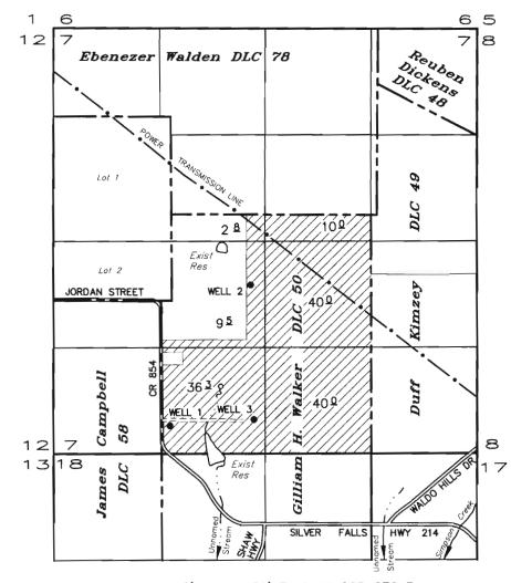
WELL 1: 425' N & 1450' E of SW COR SEC 7 WELL 2: 2100' N & 2460' E of SW COR SEC 7 WELL 3: 425' N & 2500' E of SW COR SEC 7
