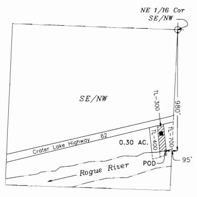
Point of Diversion - SE/NW, Section 36, T.33S, R.1W., W.M., 980 feet south & 95 feet west from the NE 1/16 corner of SE/NW, section 36
