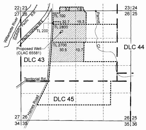
Proposed Well (CLAC 65581) is located 2,410 feet north and 2,650 feet west from the SE Corner of DLC 43.
