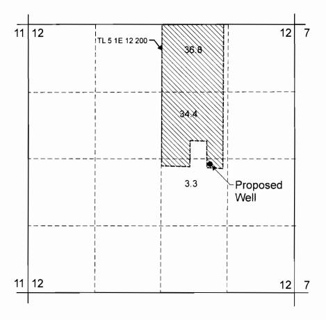
Proposed Well is located 2,750 feet south and 1660 feet west from the NE corner of Section 12.
