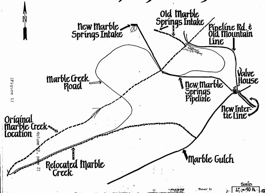
About the year of 1916 the City of Baker moved its point of diversion from the channel of Marble Creek to the "Old Marble Springs Intake." Water that was intercepted at the "Old Marble Springs Intake." is water that would have otherwise found its way to the point of diversion in the creek channel.
