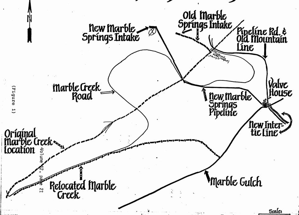
About the year of 1916 the City of Baker moved its point of diversion from the channel of Marble Creek to the "Old Marble Springs Intake." Water that was intercepted at the "Old Marble Springs Intake." is water that would have otherwise found its way to the point of diversion in the creek channel.
