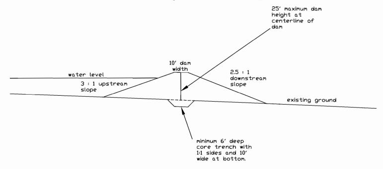
Unger Reservoir #1 will be partially dug into existing ground and partially built-up into a dike. Spillways will be located at the intersection with the natural ground level and discharged water will be diverted away from dike fill materials. Principal Spillway: Minimum 8' dia. riser conduit. Emergency Spillway: 10' wide and 2:1 side slopes.
