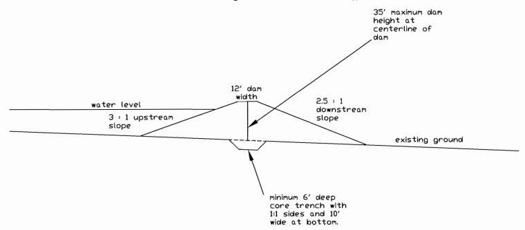
Unger Reservoir #2 will be partially dug into existing ground and partially built-up into a dike. Spillways will be located at the intersection with the natural ground level and discharged water will be diverted away from dike fill materials.
