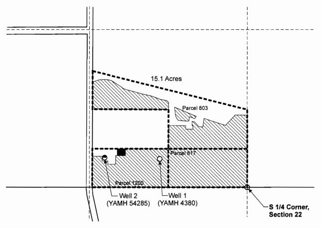
Well 1 (YAMH 4380) is located 240 feet north and 730 feet west from the S 1/4 corner, Section 22. Well 2 (YAMH 54285) is located 250 feet north and 1,190 feet west from the S 1/4 corner, Section 22.
