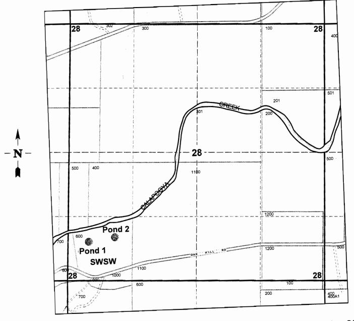
Pond 1 is located 830 ft. N. and 433 ft. E. of the SW corner of Section 28. Pond 2 is located 896 ft. N. and 981 ft. E. of the SW corner of Section 28.
