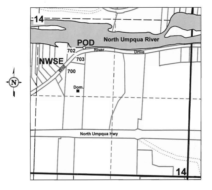
Point of Diversion is located 490 ft. South and 780 ft. East of the center of Section 14.
