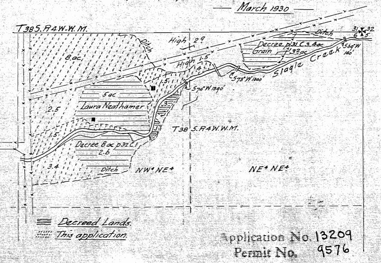
Map made by Chester Cummings by Plane Table survey in the field the same correctly showing Lands to be irrigated, to gether with disches, and streams in immediate vicinity. compiled by.
