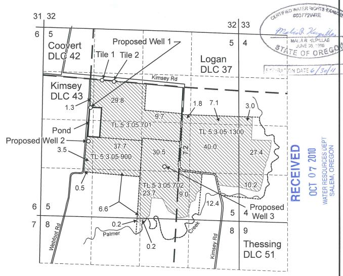
Proposed Well 1 is located 780 feet south and 0 feet west from the SE corner of DLC 42. Proposed Well 2 is located 1,690 feet south and 60 feet west from the SE corner of DLC 42. Proposed Well 3 is located 2,380 feet south and 2,009 feet east from the SE corner of DLC 42.
