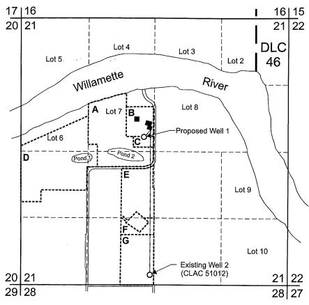
Proposed Well 1 is located 280 feet north and 2,440 feet east from the W1/4 corner, Section 21. Existing Well 2 (CLAC 51012) is located 200 feet north and 2,560 feet east from the SW corner, Section 21.
