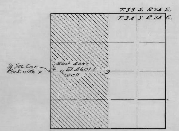
I, B.A. Martin of Brookings, Oregon do hereby certify that this map was made from notes taken during an octual survey made by me on February 14th 1956, that the monument shown on this map consisted of a Bock Marked with a cross Approximate location of well is East a distance of 400 throm the Macor Common to Sections 3 and 4 T.345. R.24 E. Wm.
