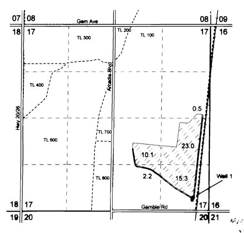
Well 1 (Malh 1860) is located 445 feet west and 380 feet north of the southeast corner of section 17.
