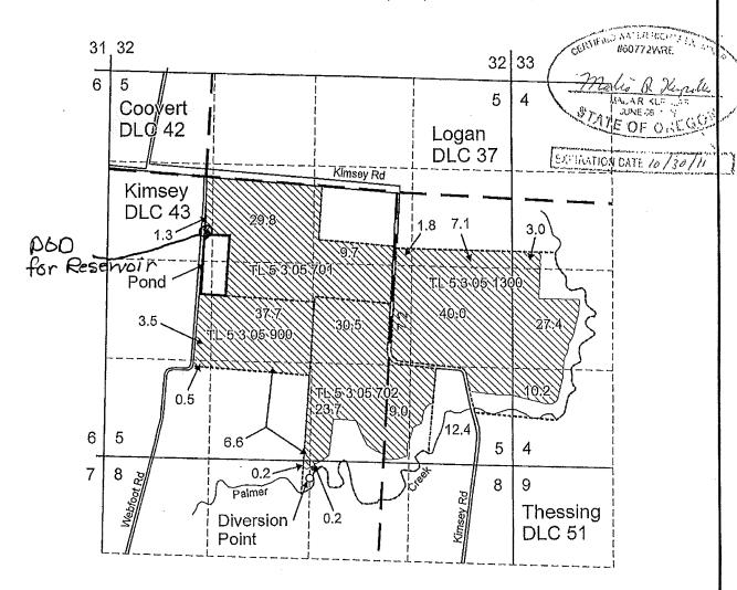
Proposed point of diversion is located 4,020 feet south and 1,350 feet east from the SE corner of DLC 42.
