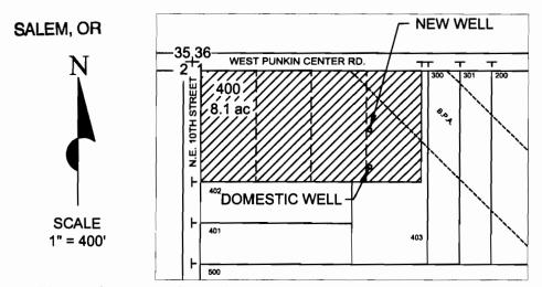
IRRIGATION WELL LOCATED 260' SOUTH & 670' WEST OF NW CORNER OF SECTION 1. DOMESTIC WELL LOCATED 400' SOUTH & 670' EAST OF NW CORNER OF SECTION 1.
