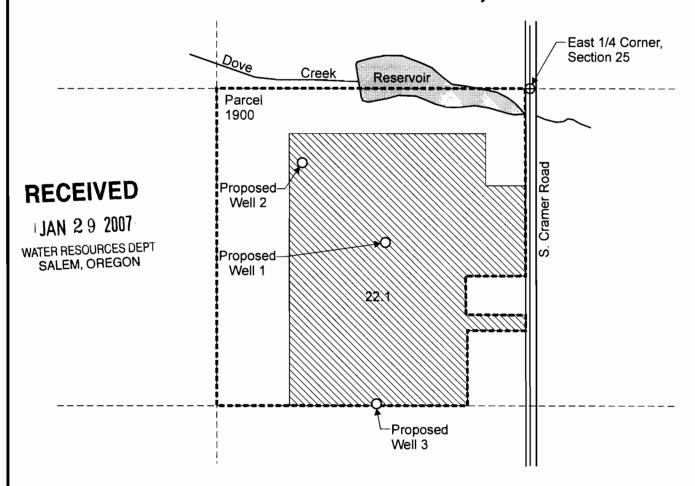
Proposed Well 1 is located 640 feet south and 600 feet west from the E 1/4 corner, Section 25. Proposed Well 2 is located 310 feet south and 950 feet west from the E 1/4 corner, Section 25. Proposed Well 3 is located 1,310 feet south and 640 feet west from the E 1/4 corner, Section 25.
