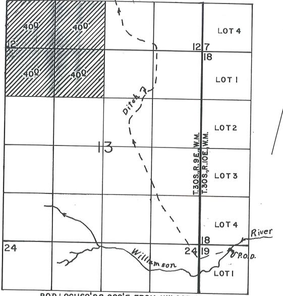
P.O.D.LOC:160'S& 800'E FROM NW COR. OF SEC 19. IN R. IOE.
