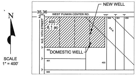
IRRIGATION WELL LOCATED 260' SOUTH & 670' EAST OF NW CORNER OF SECTION 1. DOMESTIC WELL LOCATED 400' SOUTH & 670' EAST OF NW CORNER OF SECTION 1.
